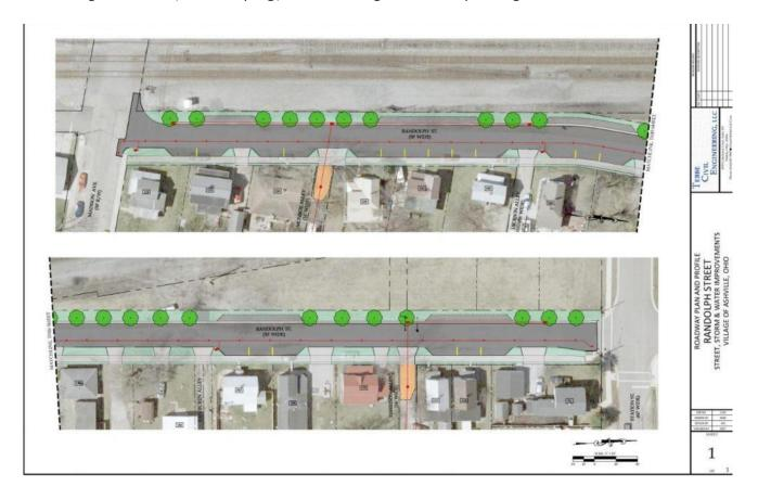
Located between Madison Avenue and West Station, the targeted area spans from 118 Randolph to 51 Station Street West. Randolph Street has suffered from significant deterioration of its roadway surface over the years, leading to considerable water runoff issues. Additionally, past pavement applications have buried the curbs, and the sidewalk on the east side is no longer visible or usable due to insufficient milling during pavement applications.
