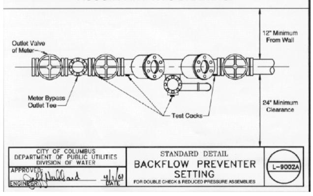
Backflow prevention assemblies shall be installed so that the inlet shut-off valve of the backflow preventor is the next piped fitting (including piping) after the water meter, except where a meter bypass, limited area fire system or strainer is needed.
